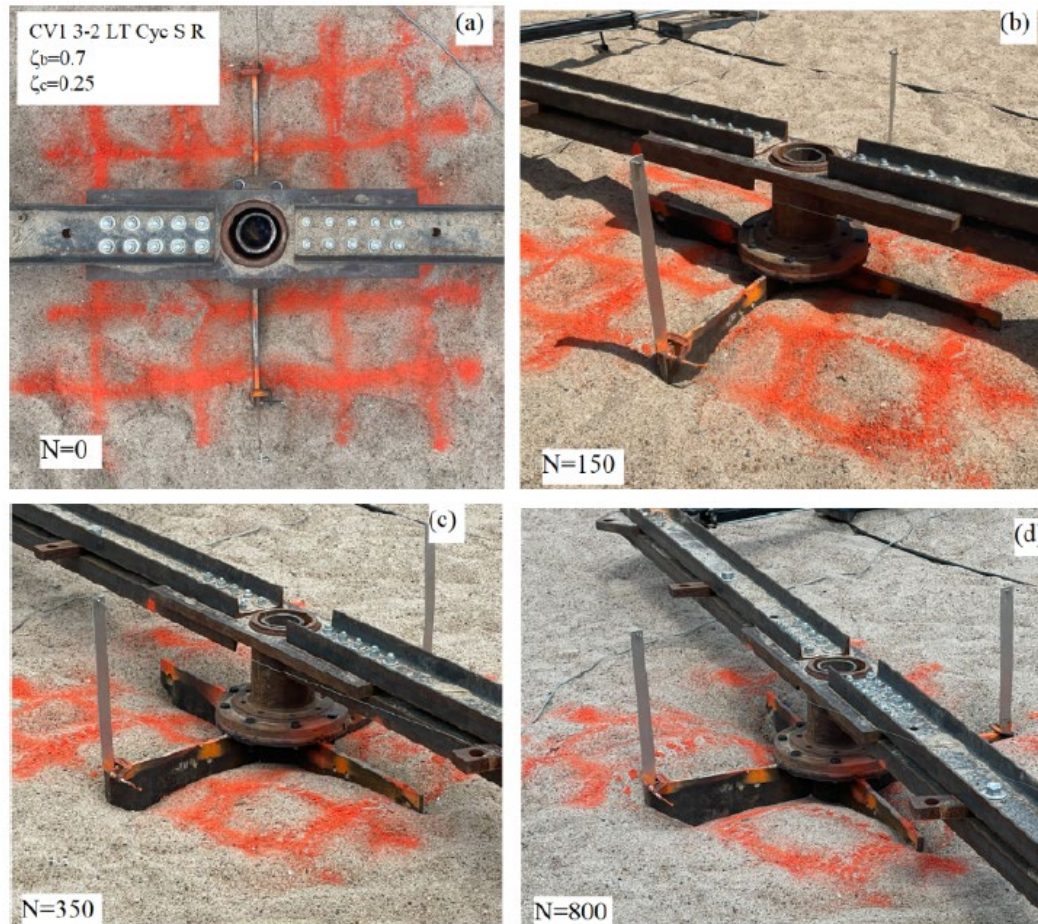
Figure 39. Soil subsidence adjacent to Collar Vane fins for CVI 3-2 during the cyclic test after a.) 0 cycles; b.) 150 cycles; c.) 350 cycles; d.) 800 cycles.
