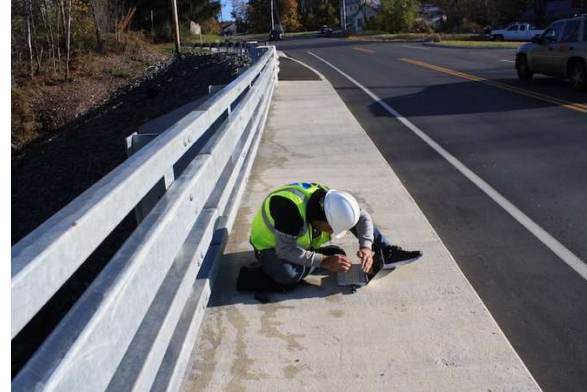
(a) Checking the condition of installed sensors. (b) Installation of an accelerometer on the bridge (c) Setup of optical sensor data collection system Figure 19. Preparation of field data collection at Grist Mill Bridge, Hampden, ME during November 3~4, 2021
