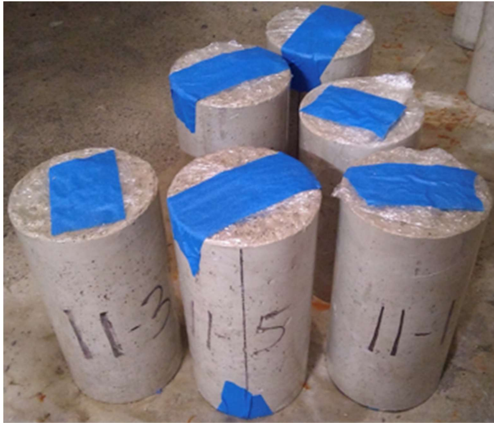
Figure 5 Sealed specimens in wet room
