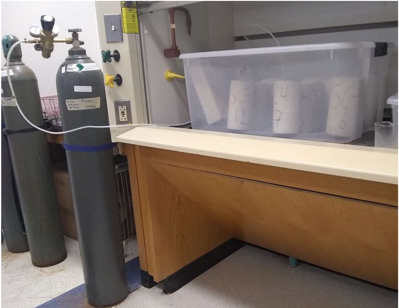
Figure 6 Carbonation Chamber Setting
