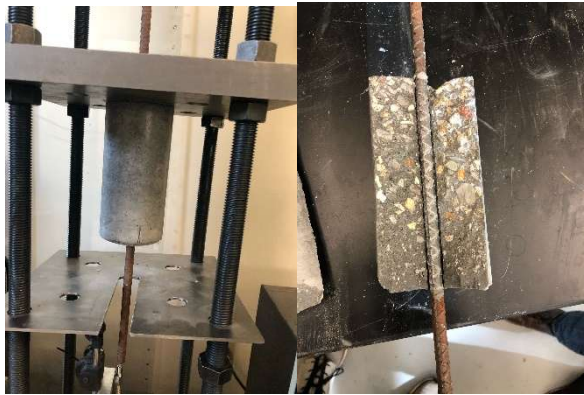
Figure 6. Pull-Out UHPC specimens with un-corroded bar.
