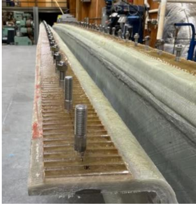
Figure 3: CT girder top flange ridges and stainless-steel shear studs
