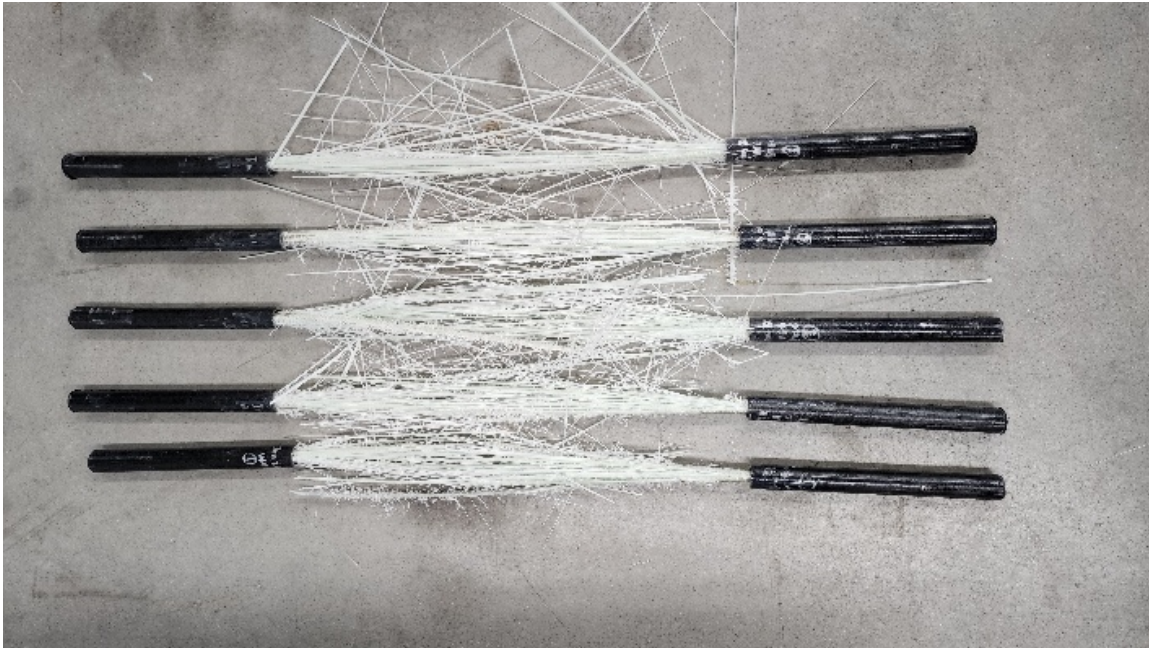
Figure 4: Failed thermoset specimens from tension tests.
