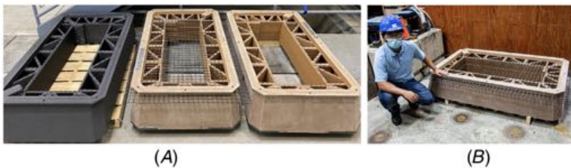
FIG. 7 Final 3D-printed formworks after postprocessing. (A) One set of CF-ABS and two sets of WF-PLA forms. (B) WF-PLA form with embedded mesh.
