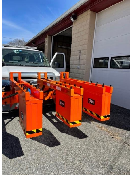
Figure 2: Three, 2 GHz antennas installed on the front of the RIDOT van
