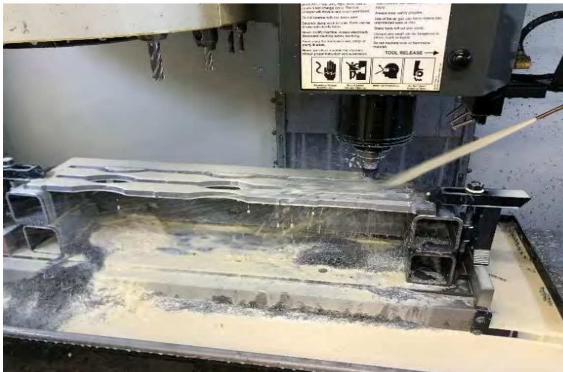
Figure 10: Fixturing of angle beams for coupon cutting
