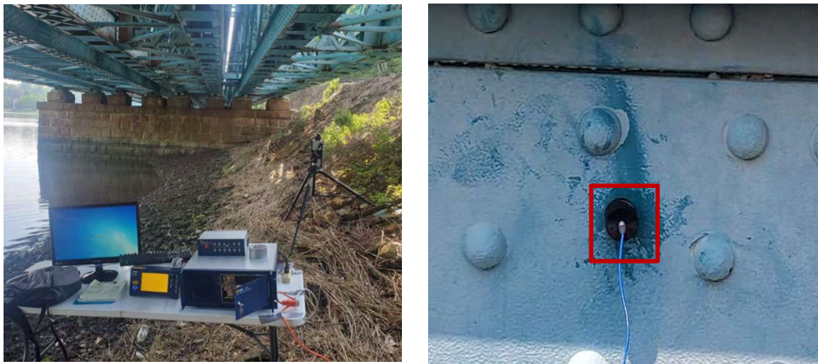
Figure 18: LDV setup to record vertical response, Laser beam pointed to node at the intersection of bottom chord and vertical members (1), Accelerometer attached to bottom chord of Cos Cob Bridge for reference (2)
