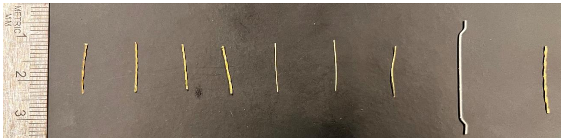
Fig. 1. Fibers with different geometries (from left to right: B2, B3, B4, B5, Straight, Striated, Wavy, Hooked and Twisted)
