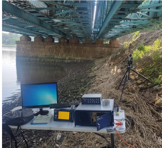
Figure 5: Laser Doppler Vibrometer (LDV) setup to record vertical displacement of the bridge during train traversal.
