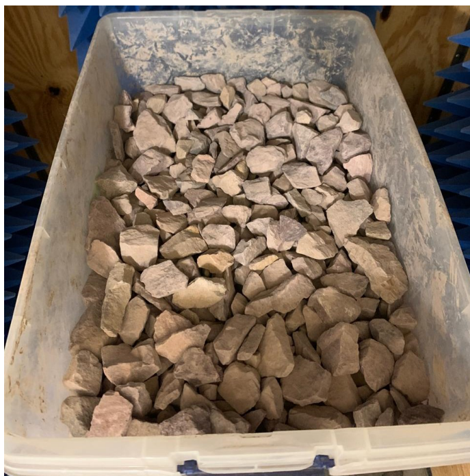
Figure 3: Ballast aggregates and fine silty sand (fouling) materials used in experiments
