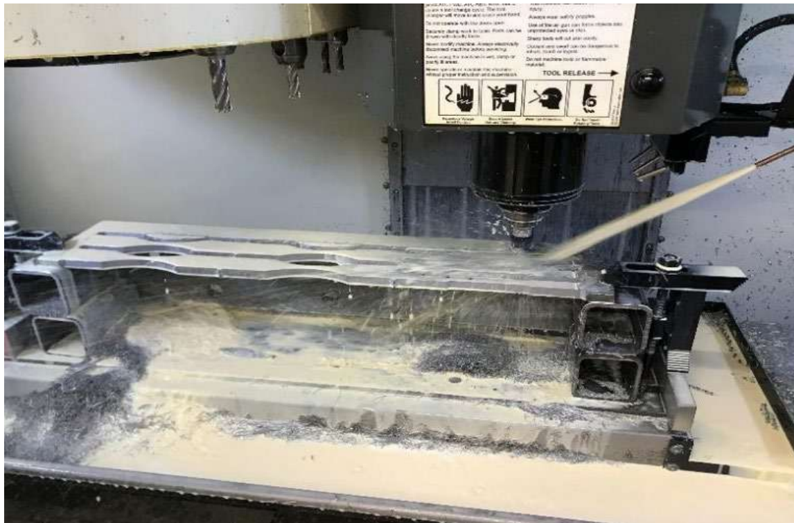
Figure 10: Fixturing of angle beams for coupon cutting
