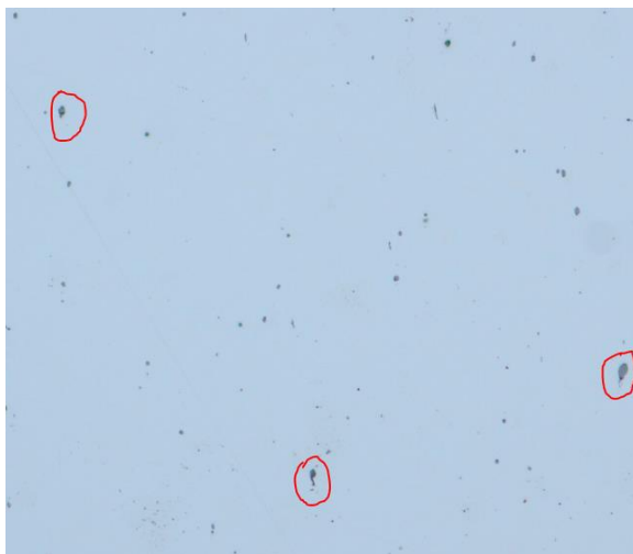
Figure 1 – Microstructure image of Devon, bridge (CT) sample material, encircled in red are MnS intrusion
