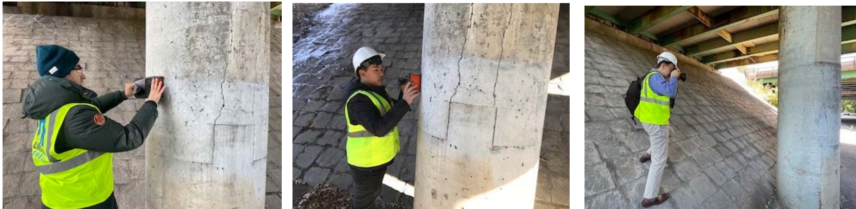
Figure 1. (a) GPR inspection of corroded RC bridge pier column (Koosha and Nak); (b) Visual inspection of RC bridge pier column (PI Yu)
