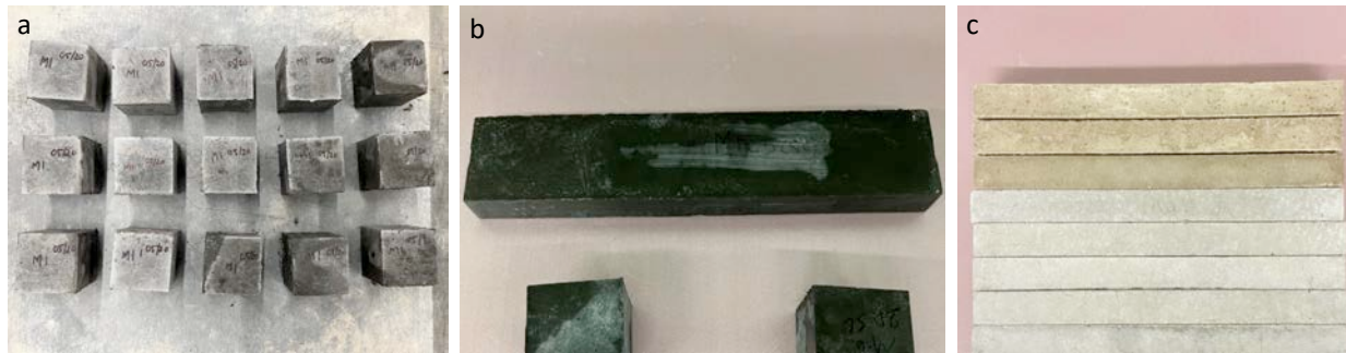
Figure 2. (a) cubes for compressive strength test, (b) beams for flexural strength test, and (c) mortar bars for ASR expansion test.
