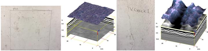
(a) Intact surface and its radar image
