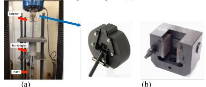
Figure 3: (a) Apparatus of pull-out test and (b) different types of grippers for the pull-out test.
