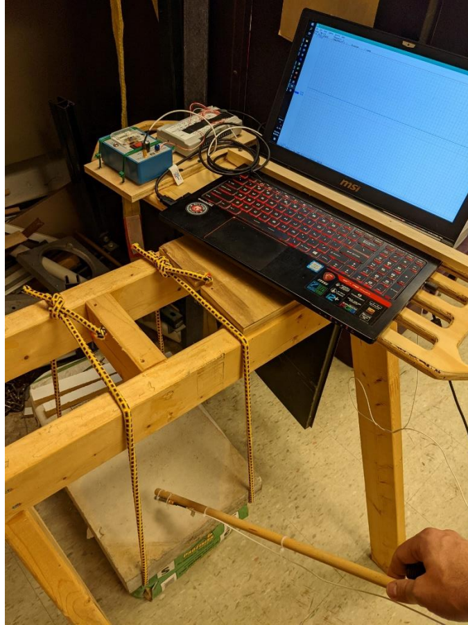
Figure 1. Testing of concrete delamination phantom with acoustic sensor arm and portable data acquisition system.
