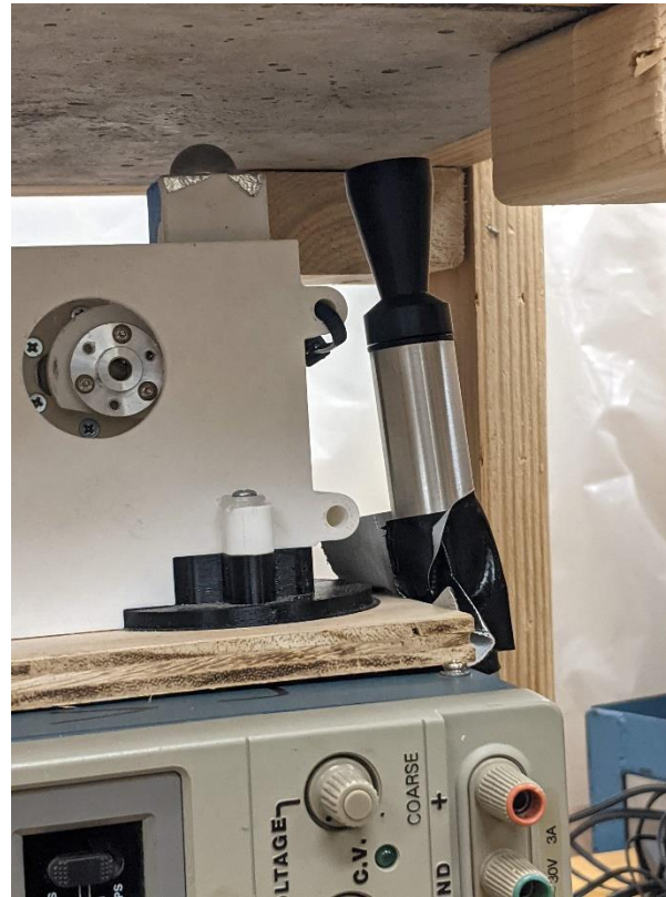
Figure 2. Close up of acoustic sensor arm with digital microphone in laboratory slab test setup
