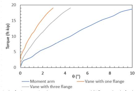
Figure 1. Angle of twist comparison between moment arm and CV flanges. Results for the CV36-36.
