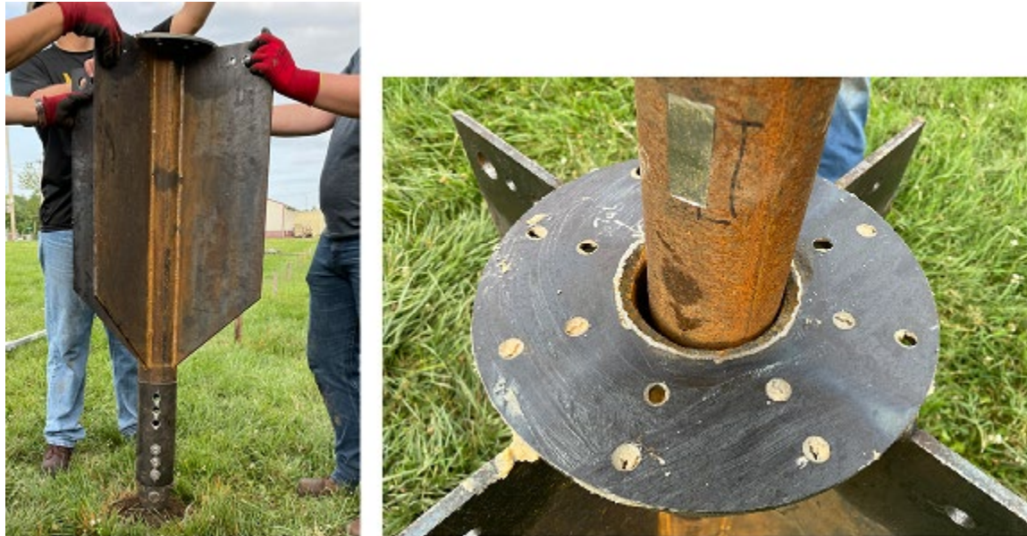
Figure 3. Single-piece collar vane implemented in summer 2022 testing plan. (a) Collar Vane installation. (b) Detailed top flange where all the 4 blades are connected to it.
