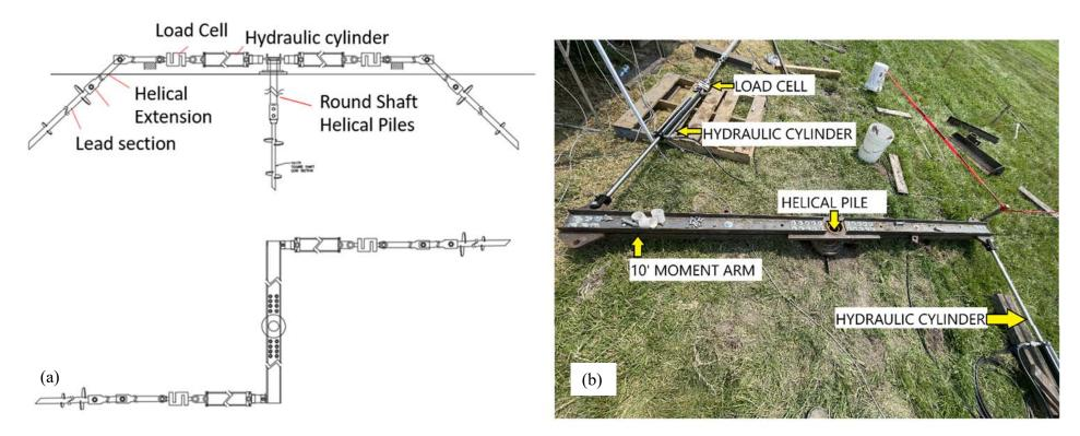
Figure 1. (a)Test frame schematic for torsion test (b) Actual test frame for torsion test.
