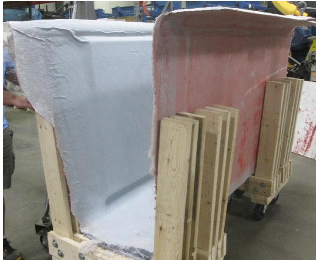
Figure 1: Completed Mock-Up Section of Girder
