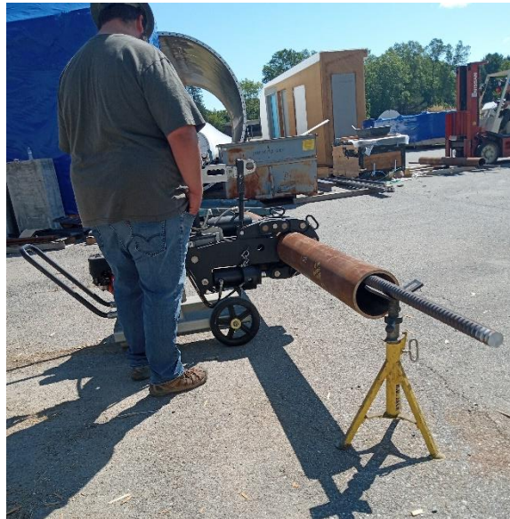
Figure 1 Specimen assembly process: Application of makeup torque to the steel casing.
