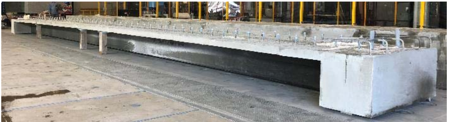
Staged Strength Testing Girder Specimen
