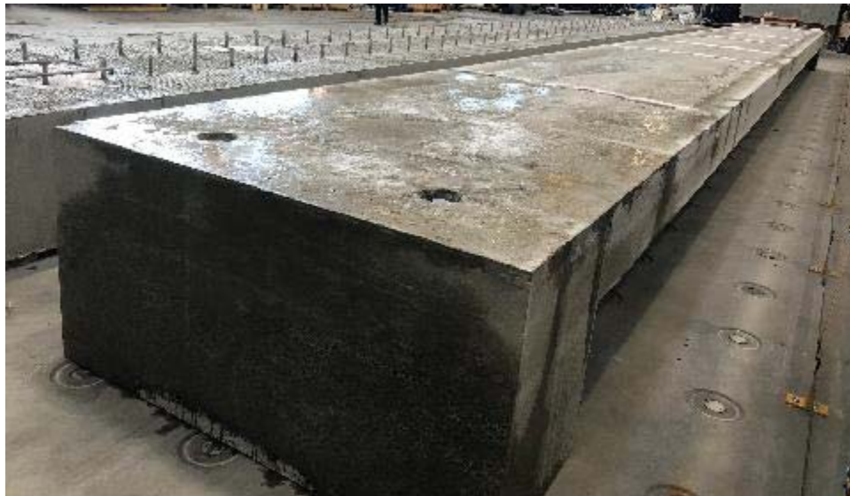
Creep Testing Girder Specimen
