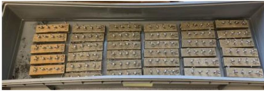
Figure 2. Chloride penetration testing of concrete specimens with various loadings of shrinking fibers: a. specimens soaking in saline bath, b. specimen with embedded electrodes for Wenner probe testing.
