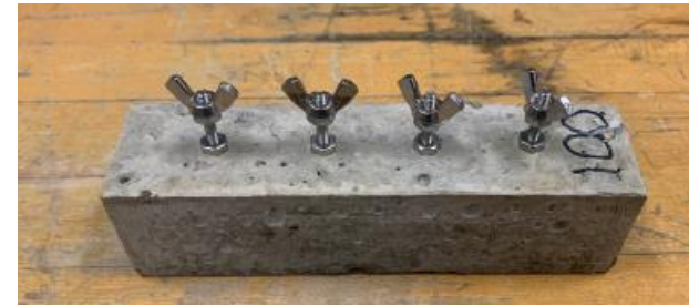
Figure 2. Chloride penetration testing of concrete specimens with various loadings of shrinking fibers: a. specimens soaking in saline bath, b. specimen with embedded electrodes for Wenner probe testing.
