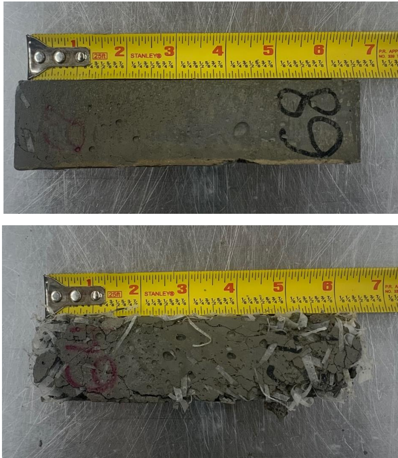
Figure 2. After 168 freeze-thaw cycles; 0.24 wt% active fiber specimen with minimal damage (top) and 2% passive fiber specimen with significant damage (bottom)
