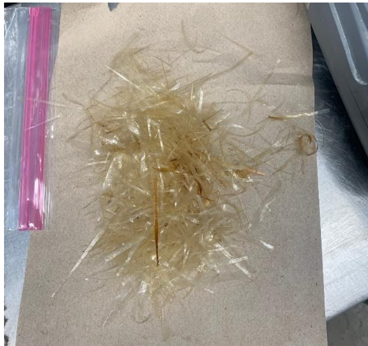
Figure 1. Chitosan fiber produced by improved manufacturing technique
