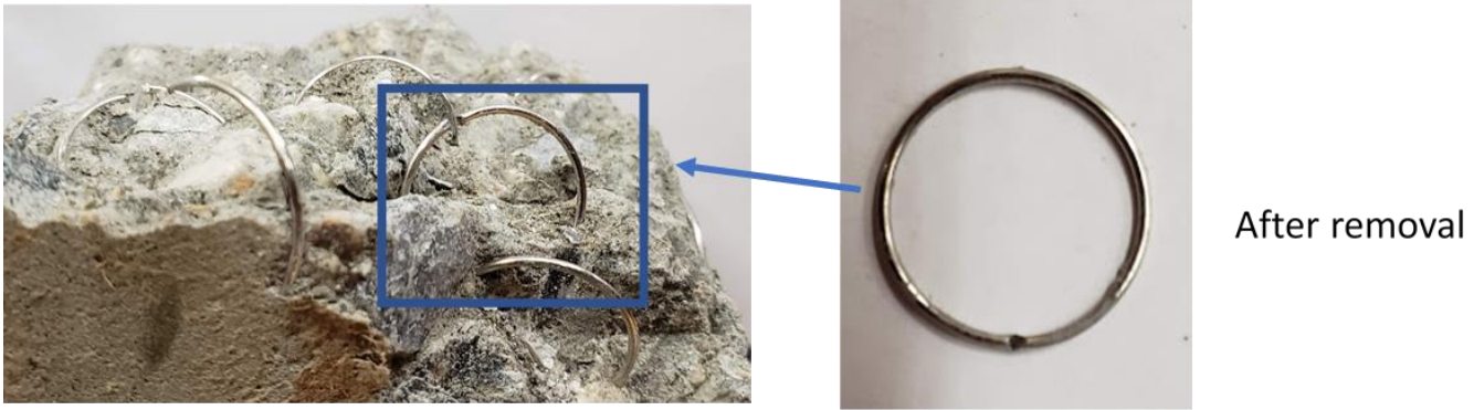
Figure 3. The ring is deformed when imbedded in the beam, but returns to its original shape after removal from the concrete matrix. This confirms that the rings set into the concrete in a deformed prestressed state following dissolution of the PVA.
