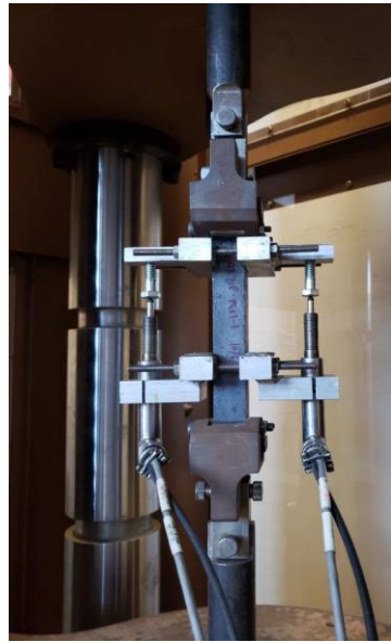
Fig:- Direct Tension Test Setup
