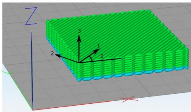
Material deposition direction in 3D printing.
