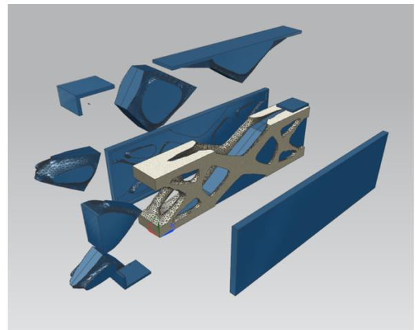
Figure 5: 3D printed forms (in blue) for topology optimized precast concrete diaphragm
