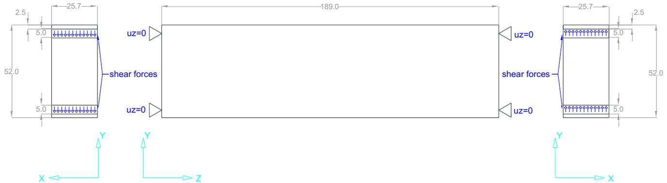
Figure 4: Dimensions, loading (for load case I) and boundary conditions for a prismatic diaphragm used for topology optimization.
