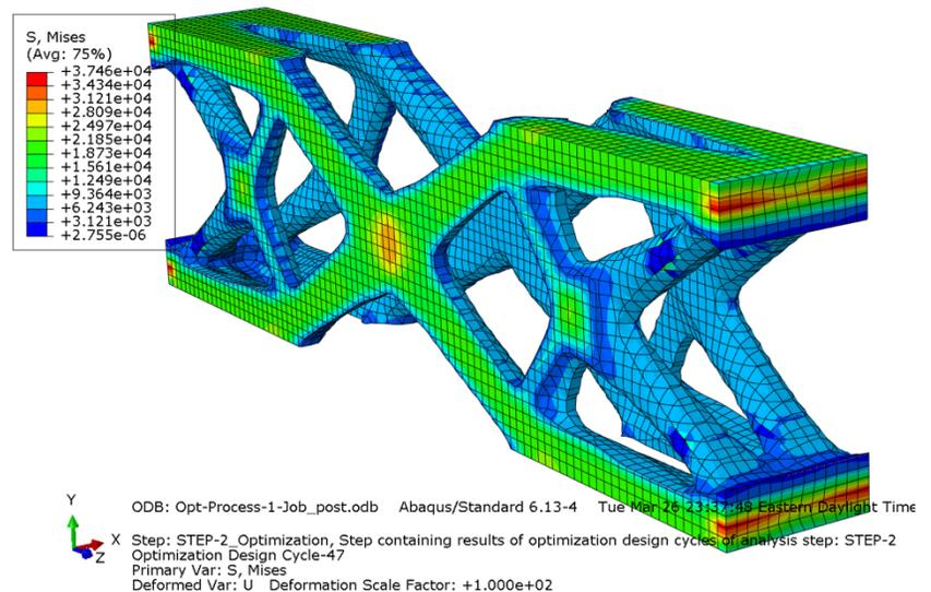
Figure 3: Topology optimized geometry obtained after 50 iterations
