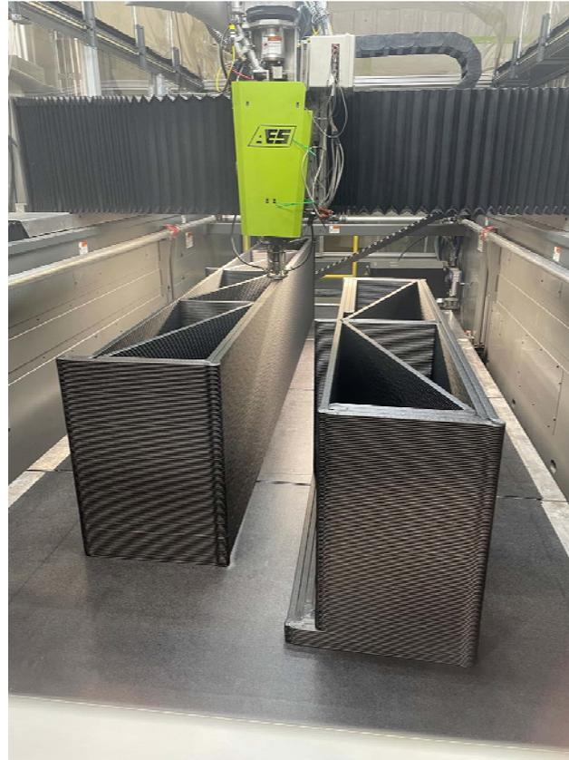
*Figure 2 – Railroad bridge ballast retainer 3D printed forms for American Concrete Industries, Veazie, ME*
