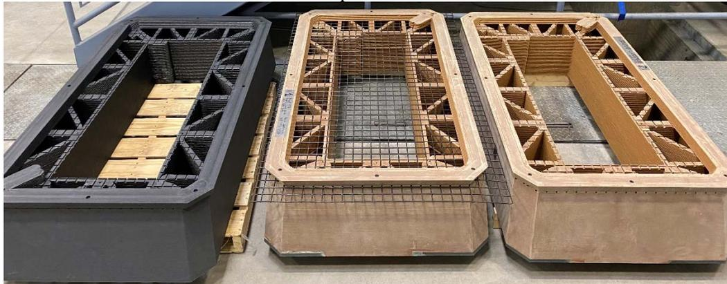
*Figure 1 – 3D printed formwork sets with three different polymer composites for Unistress Corp., Pittsfield, MA*
