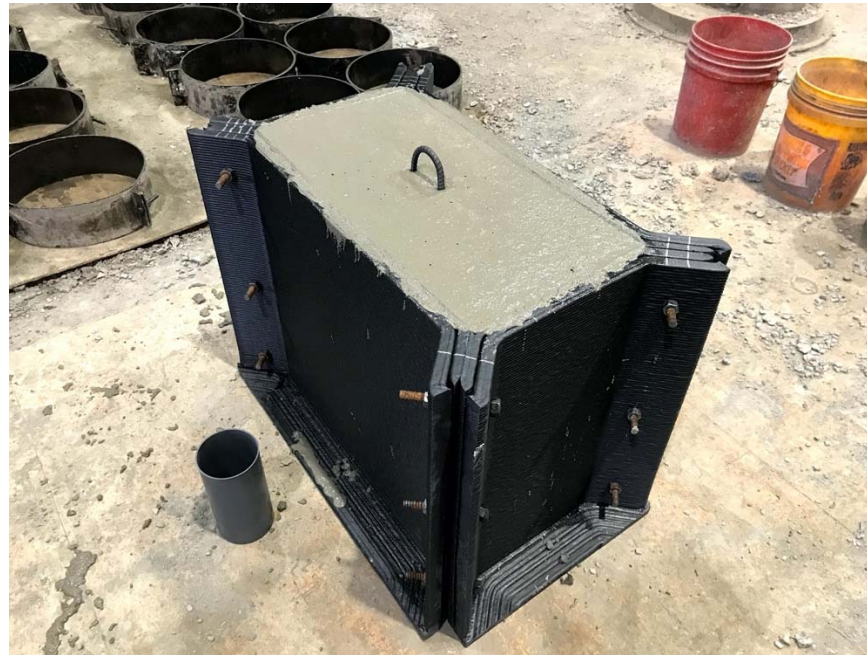
Figure 1 – 3D printed formwork prototype after casting concrete
