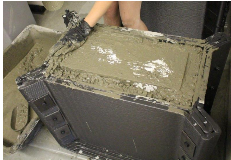
Figure 1 – Concrete casting in CF-ABS formwork
