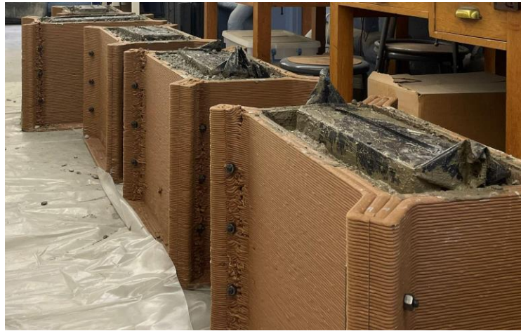
Figure 2 – Cast and assembled WF-aPLA formwork
