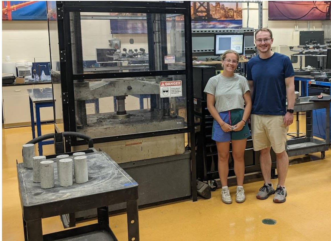
Figure 2 Concrete test cylinders with various amounts of ground glass pozzolanic cement undergoing compression testing
