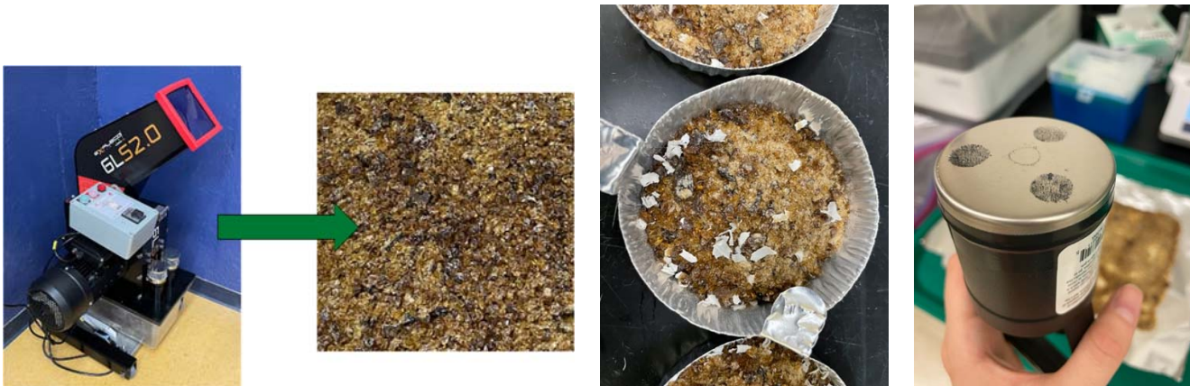
Glass crusher and lab manufactured processed glass aggregate (LM-PGA), LM-PGA samples post-furnace process, metal collected from LM-PGA
