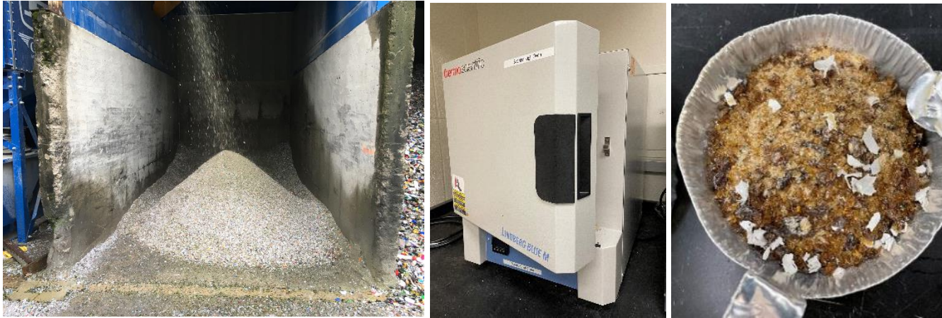
PGA produced at the CSWD facility; 550 deg furnace; furnace test lab-manufactured sample
