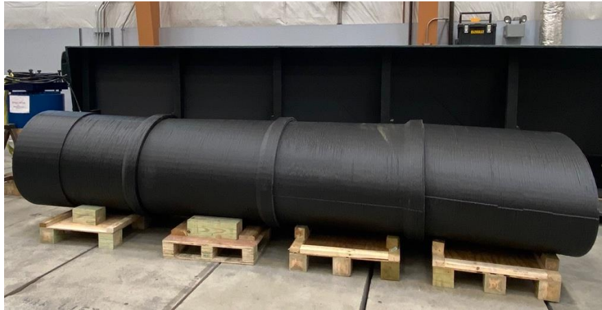
Figure 2. Pre-assembled 3D printed culvert outlet diffuser segments.
