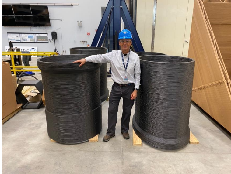
Figure 1. 3D printed culvert outlet diffuser segments.
