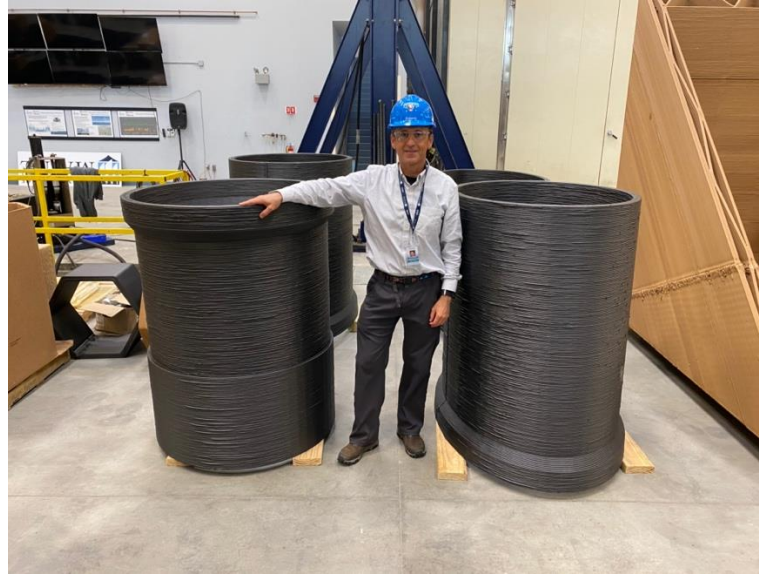
Figure 1. 3D printed culvert outlet diffuser segments.
