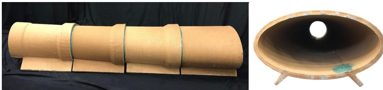
Figure 4: Side view and end view of assembled 3D printed culvert diffuser
