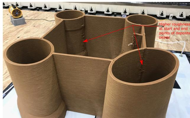
Figure 3: 3D printed culvert segment.
