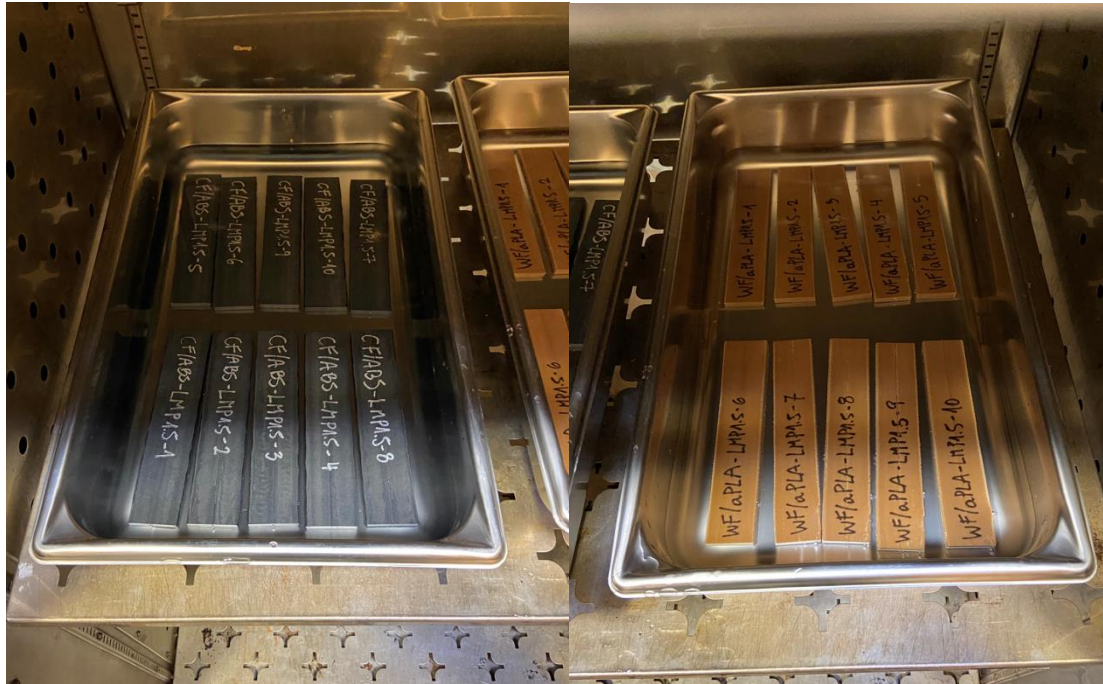
Figure 1. CF/ABS and WF/aPLA specimens immersed in water for moisture conditioning.
