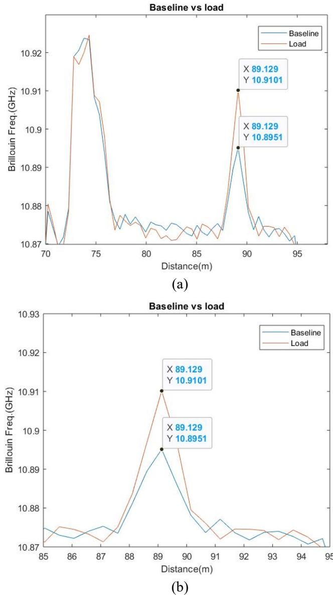
Figure 9. BOTDR results for the sensing fiber cable area.
