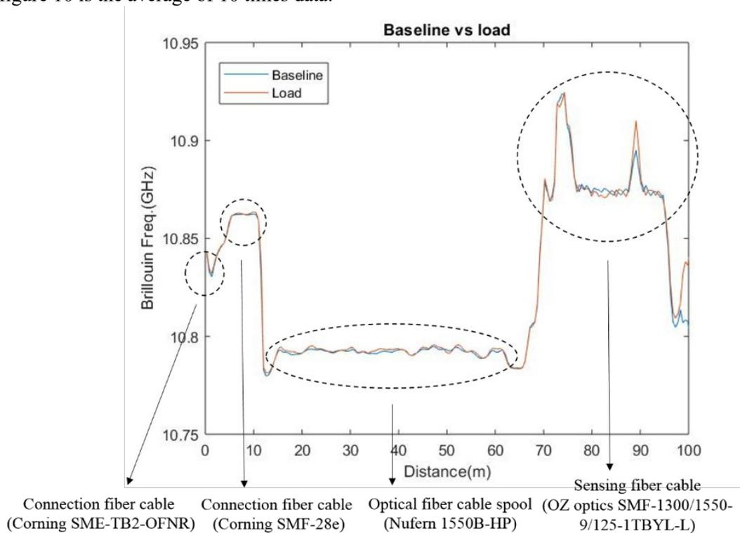
Figure 8. BOTDR results for the entire connected fiber cable area.
