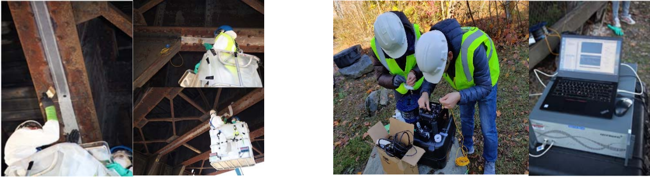
Figure 3 Attaching optical sensor with epoxy and connecting sensor to BOTDR
