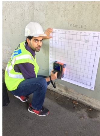
(b) Field radar imaging at Lincoln St. Bridge (Lowell, MA) (Left: Grad. RA: A. Alzeyadi / Right: Grad. RA: H. Gandhi)
