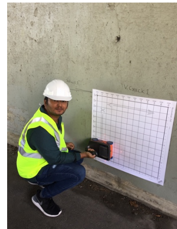
(b) Field radar imaging at Lincoln St. Bridge (Lowell, MA) (Left: Grad. RA: A. Alzeyadi / Right: Grad. RA: H. Gandhi)
