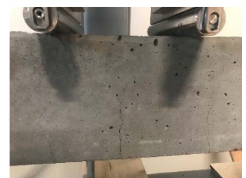
Fig. 1 c) Cracks generated
