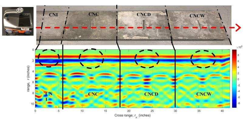
In the last report, we provided the information on series of image processing techniques to detect the crack in artificially cracked specimens CNI, CNC, CNCD and CNCW using the 1.6 GHz portable ground penetrating radar (GPR). In this report, we formulate the mathematical model to calculate the depth of an artificial crack on concrete panels. Fig. 1 shows the 1.6 GHz GPR and the B-scan GPR images of intact and artificially-cracked
