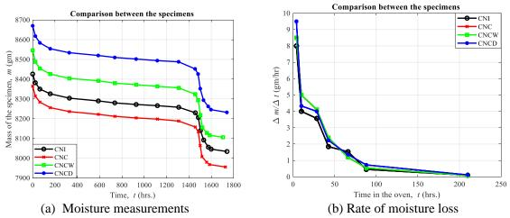
Figure 1. Time-dependent variations of moisture level in all four concrete specimens for approximately three months
