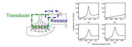
This figure illustrates the basic mechanism of the non-contact sensor as well as the impedance measurement. The modeling of the sensing measurement has been established. Parametric analysis has been conducted to elucidate basic design criteria of the sensory system to acquire impedance measurement for damage identification.
