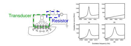
This figure illustrates the basic mechanism of the non-contact sensor as well as the impedance measurement. The modeling of the sensing measurement has been established.
