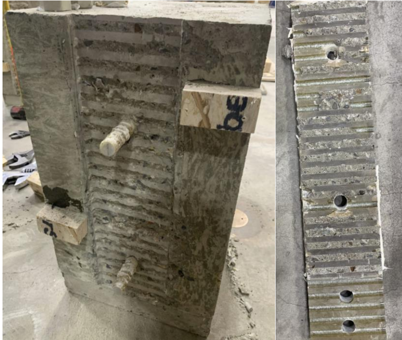
Figure 36: Specimen 5 – Side A Heavy Damage (Left: Concrete, Right: FRP)
