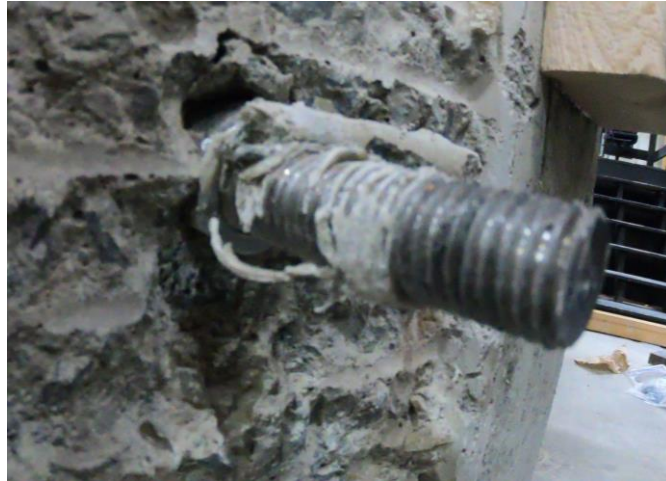
Figure 31: Specimen 4 – Stainless Stud Yielding and Pullout
