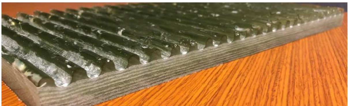
Figure 2: Ridged FRP Shear Connection
