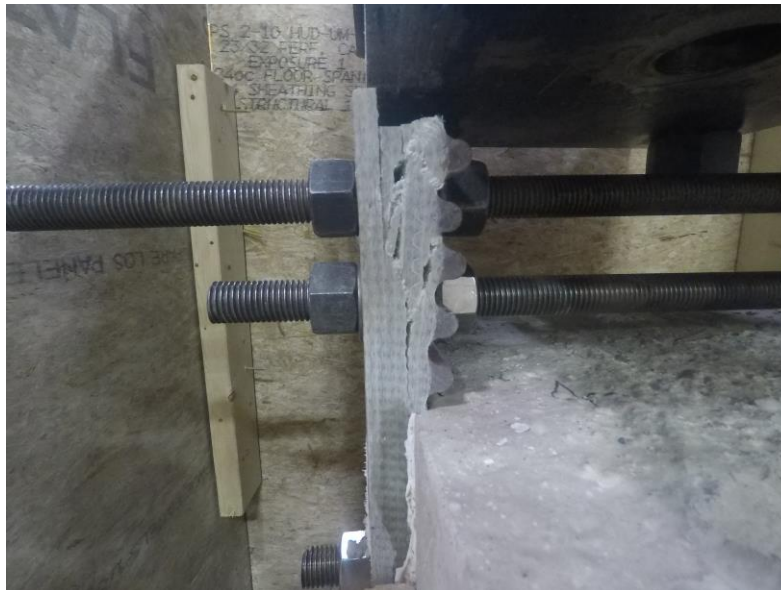
Figure 28: Specimen 3 – FRP Crushing
