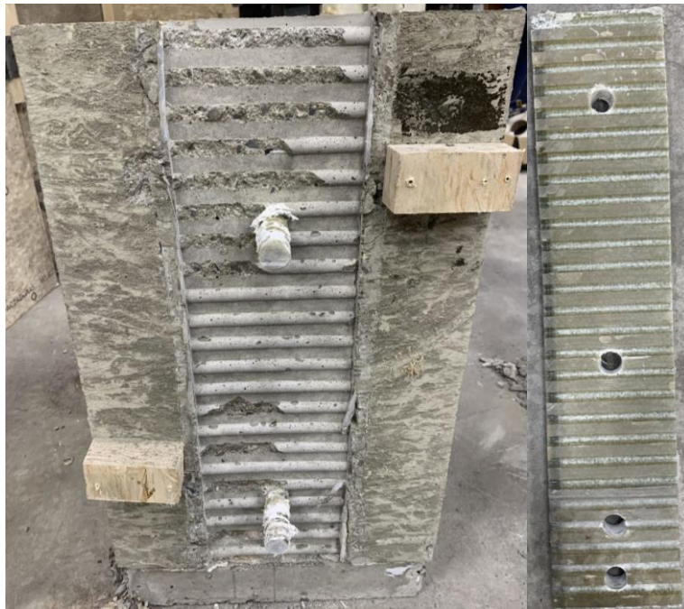
Figure 37: Specimen 5 – Side B Moderate Damage (Left: Concrete, Right: FRP)
