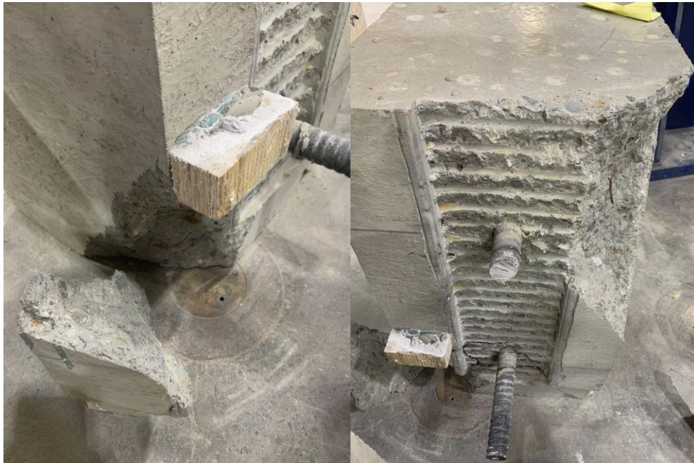
Figure 22: Specimen 2 – Concrete Crushing Failures
