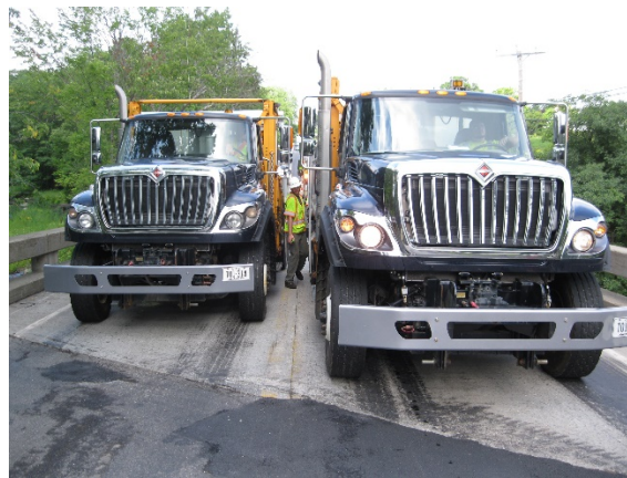
Figure 1: Skewed T-Beam Bridge Live-Load Testing
